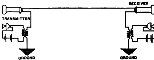
FIG. 353.— Illustrating the connections of a telephone circuit during conversation.
